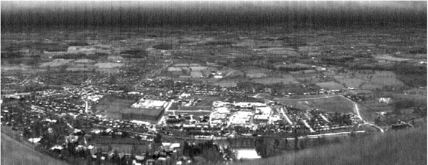
Figure 1. Passive mm-wave image looking east from the Malvern Hills illustrating the natural imagery provided by passive mm-wave imaging.
