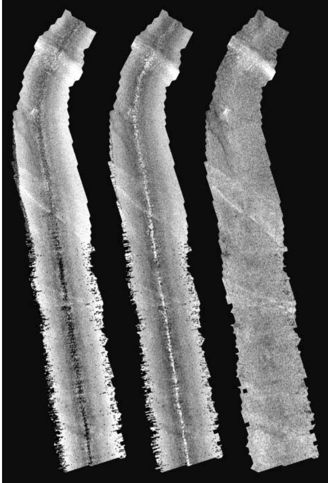
Fig. 6: Top view render of bathymetry mesh with different texture maps. From left to right: unprocessed backscatter image, restored backscatter by standard linear interpolation and restoration using the proposed method.
