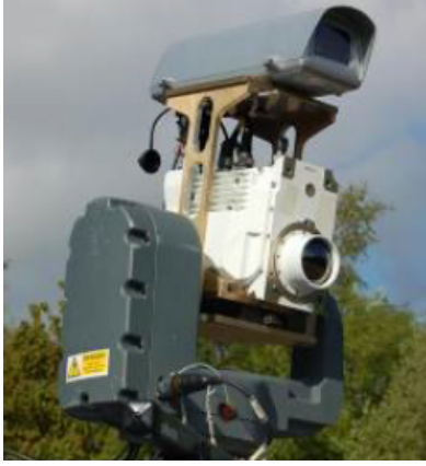
(a) Jai's AD-080 GE (upper) and Thales' Catherine MP (lower) mounted on a pan & tilt head.
