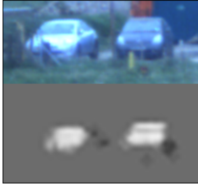
Figure 2: Emitted radiation is partially polarised in a plane perpendicular to the surface, and polarisation is strongest for surfaces observed near grazing angle. An image of two vehicles is presented as observed in the Q Stokes image (upper) and the visible (lower). Notice that the roof is present with maximum intensity, and the sides are present with minimum intensity.
