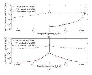
Fig. 7. Normalized Doppler PSDs of the proposed adaptive model for different SISO pico-cell scenarios ( $\delta_T = \delta_R = 0, \chi = 0$ ): (a) Tx and Rx move in opposite directions, (b) Tx and Rx move in the same direction. VTD: vehicular traffic density.
