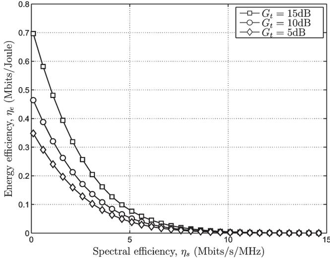
Fig. 3. EE-SE relation considering only the transmit power in the CRNs.
