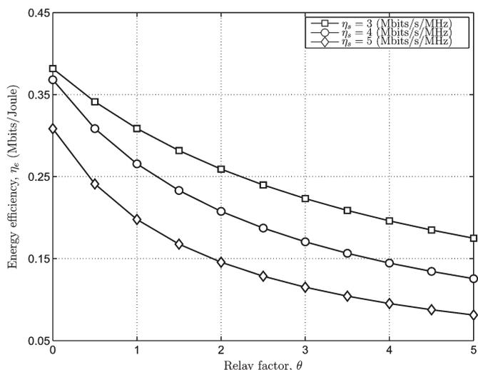
Fig. 7. EE of the OCRNs against the relay factor  $\theta$  with varying SEs.
