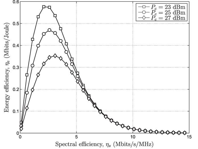
Fig. 4. EE-SE relation in a practical CRN with varying circuit powers  $P_c$ .
