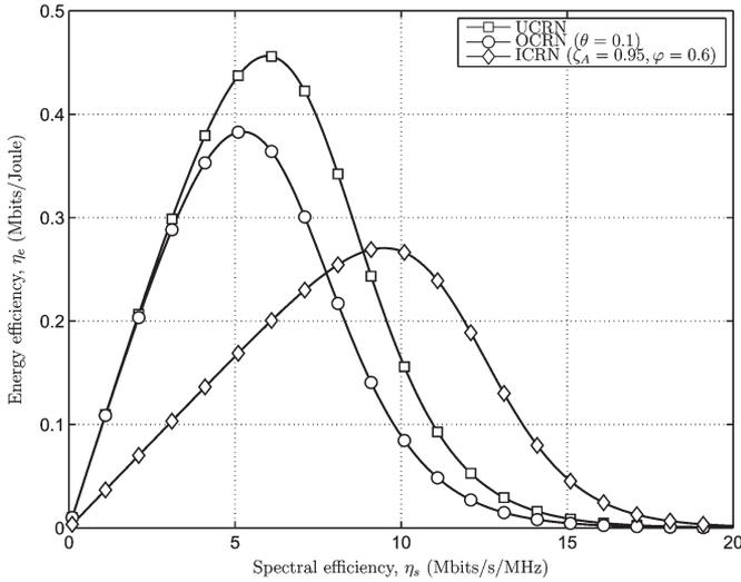
Fig. 9. EE-SE relation for three CRNs: the UCRNs, the OCRNs, and the ICRNs.
