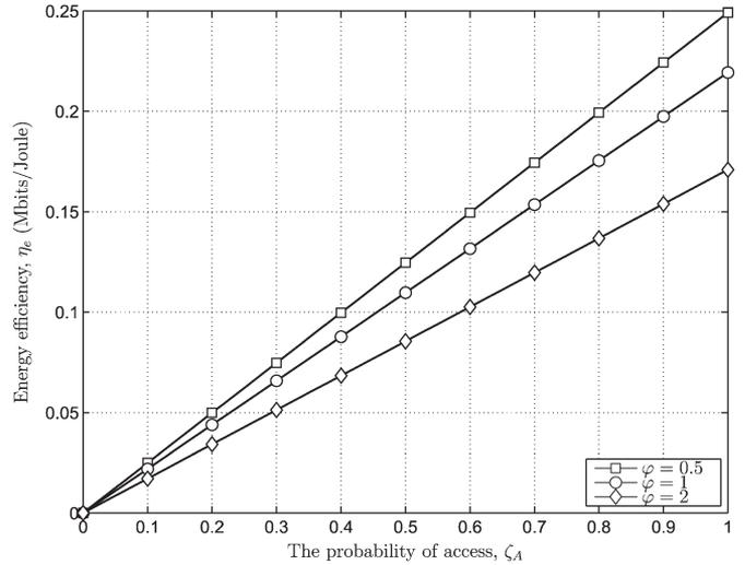
Fig. 10. EE in the ICRNs against the probability of access with varying sensing factors  $\varphi$ .
