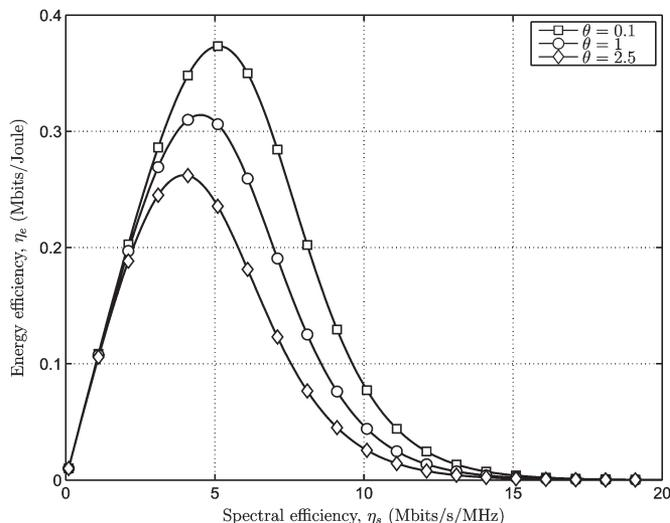
Fig. 6. EE-SE relation in an OCRN with varying relay factors  $\theta$ .
