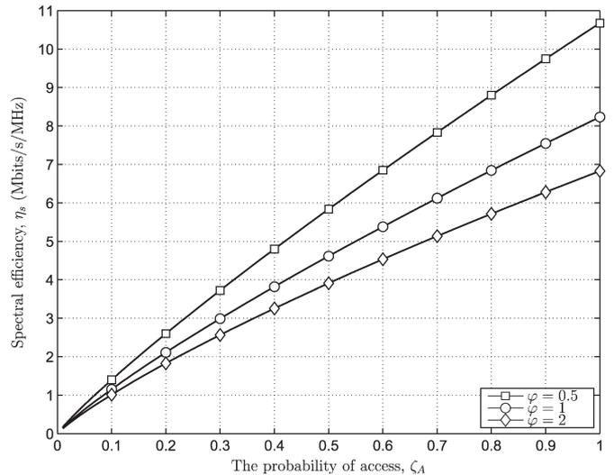
Fig. 11. SE in the ICRNs against the probability of access with varying sensing factors  $\varphi$ .
