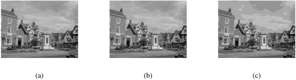
Figure 3: (a) The original image, (b) Standard Q50 JPEG compression, (c) Our new visually interesting region compression: Q50 in top 40% visually interesting regions, Q5 elsewhere. Note by inspection that the visually important regions in the image are generally preserved, while the contextual information outwith the core remains valuable, although highly degraded. The compression ratio is improved from 5.25 \pm 0.5 to 6.0 \pm 0.3 using our method without loss of detail at the salient locations (in this case the house).
