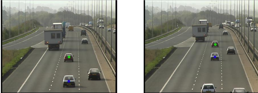
Figure 12: Tracking the centroid of a contour using a Kalman estimate, first and last images in sequence
