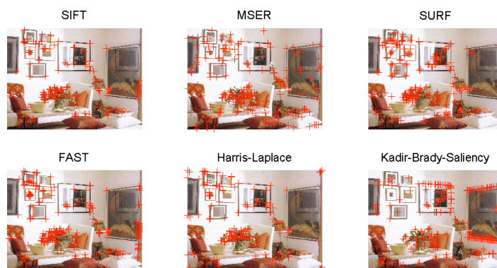
Fig. 1. An illustration of distribution of the interest-point detectors used in this paper.
