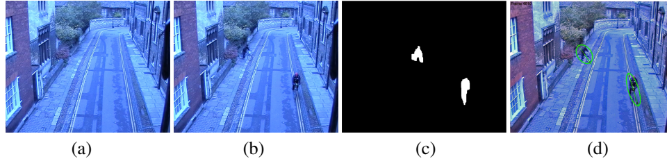
Figure 1.1 Automatic initiation of targets using background subtraction is possible when the camera is static.
