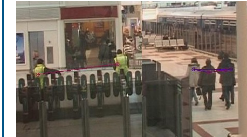
Result: Image plane tracks with the scene segments. Green tracks are in the traffic region, and blue in idle areas.
