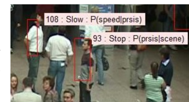
Example 1: We found that we are able to detect the true positive instances of globally unusual behaviour. In this instance running through the scene was identified as an abnormal behaviour. High speeds have a low statistical representation for all scene segments and thus are detected as the individuals run through multiple scene segments
