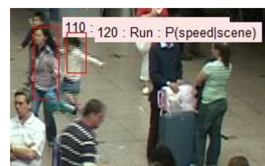
Example 1: We found that we are able to detect the true positive instances of globally unusual behaviour. In this instance running through the scene was identified as an abnormal behaviour. High speeds have a low statistical representation for all scene segments and thus are detected as the individuals run through multiple scene segments
