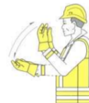
Fig. 1: An illustrative gesture from the current EU guidelines: a “move forward” command [7]
