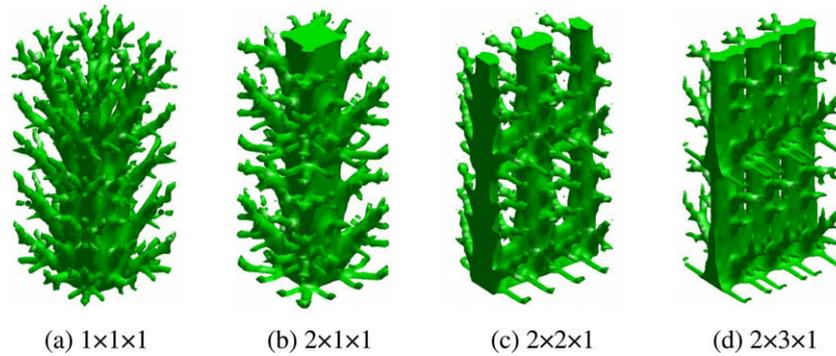
Fig. 4. Full conductivity designs for periodic structures without thermoelastic coupling.
