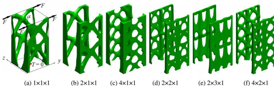
Fig. 3. Full stiffness designs for periodic structures without thermoelastic coupling.
