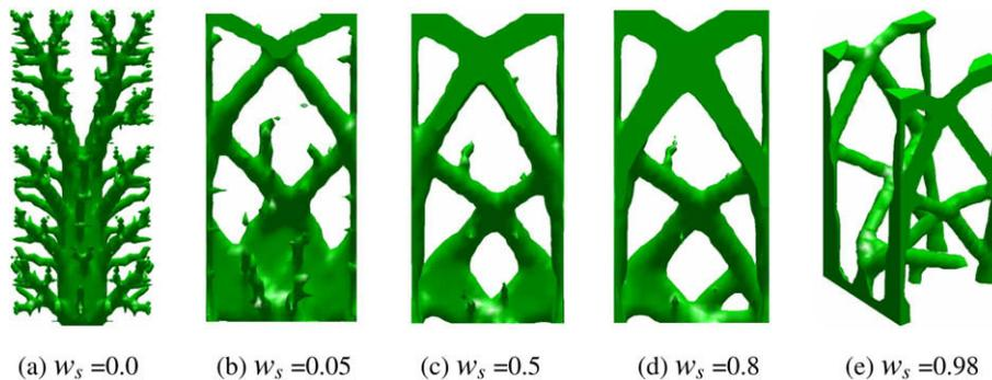
Fig. 7. Periodic structural designs with increasing stiffness weight (thermoelastic coupling).
