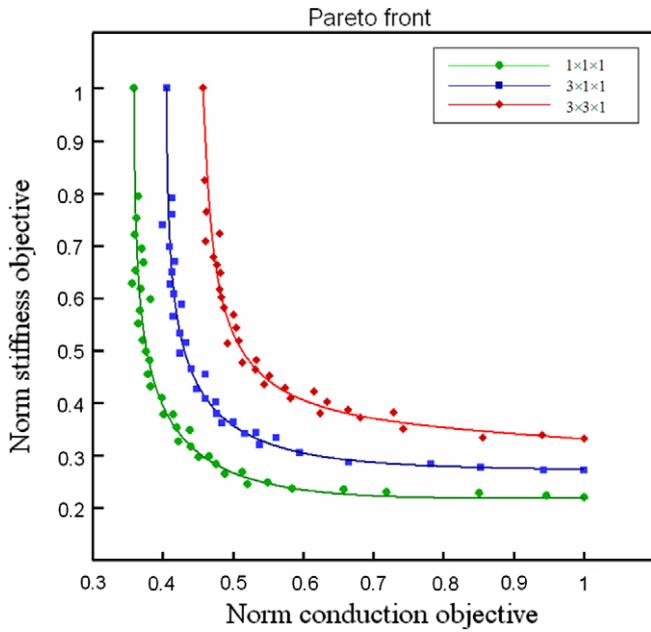
Fig. 6. Pareto fronts of different periodic structures (without thermoelasticity).
