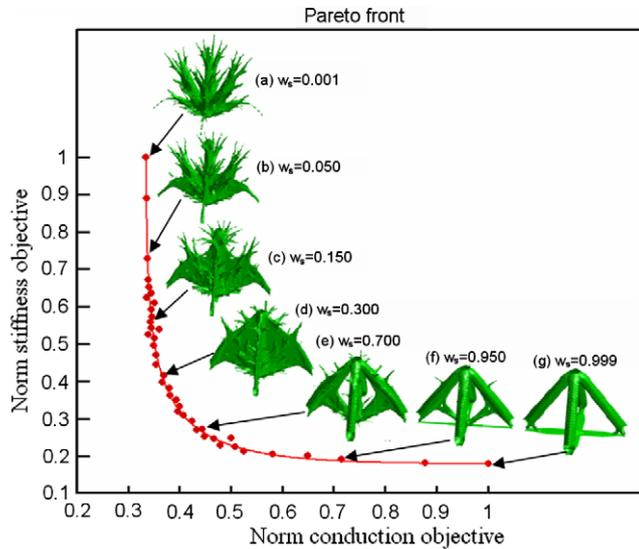
Fig. 2. Pareto front and corresponding structural topologies.
