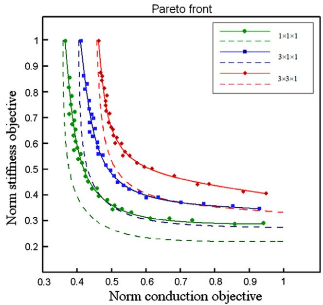
Fig. 8. Pareto fronts for finite periodic structures with thermoelastic coupling. Dashed curves indicate the Pareto fronts without thermoelasticity.
