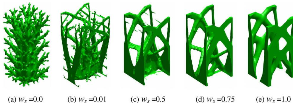
Fig. 5. Periodic structural designs with increscent stiffness weighting factors (without thermoelasticity).
