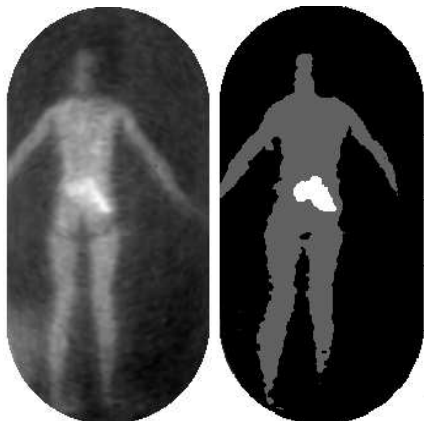
Figure 4: Expectation-Maximisation segmentation (right) of a scene containing a potential target in a MMW image (left).
