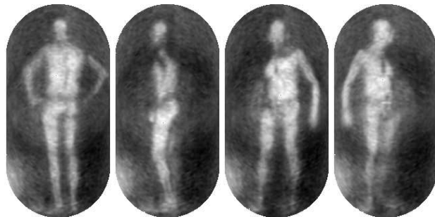
Figure 1: Example MMW image showing a human subject. Notice the Speckle noise pattern particularly apparent on the torso and the substantial smoothing which is applied during the image formation process to minimise visual artifacts.
