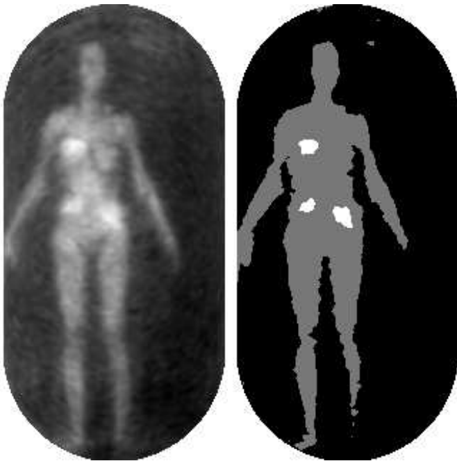
Fig. 4 Expectation-Maximisation classification (right) of a scene containing potential targets in a MMW image (left). The subject is carrying three small metal objects and the classification performs well in this example.
