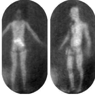
Fig. 6. Two example frames showing where the metallic threat object can be identified solely from the intensity (left) and where only the shape of the object identifies the threat (right - threat is on the subjects right hip).
