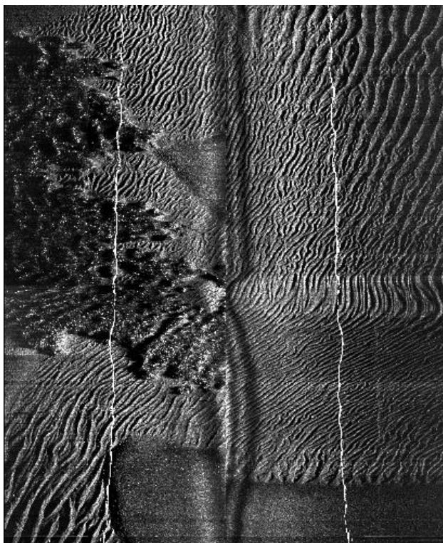
Fig 9 A raw Sidescan image containing regions of flat, rippled and complex seafloor.
