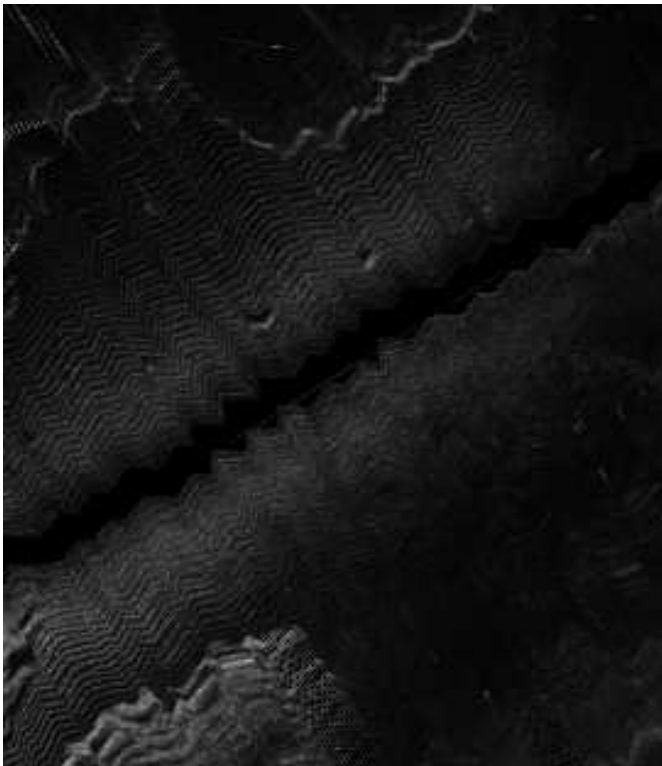
Fig. 5. A geo-referenced side-scan mosaic created using the AUVs output.
