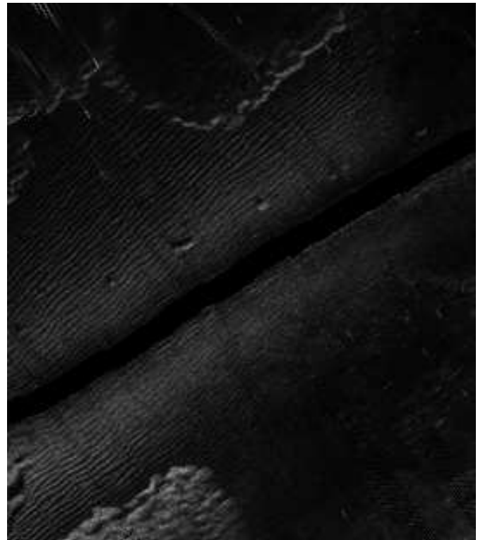
Fig. 6. A geo-referenced side-scan mosaic created using a Kalman-RTS system.
