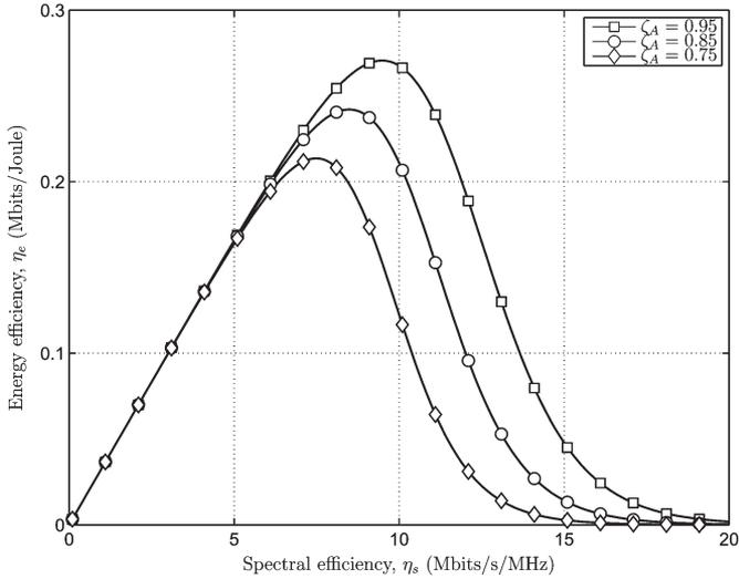
Fig. 8. EE-SE relation in the ICRNs with varying probabilities of access  $\zeta_A$ .
