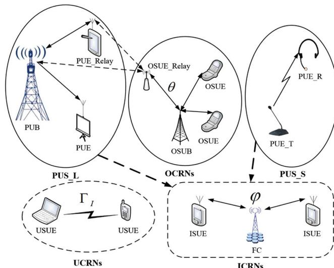
Fig. 1. General coexistence model between PU systems (large- and small-scale PU systems) and three CRNs (UCRNs, OCRNs, and ICRNs).
