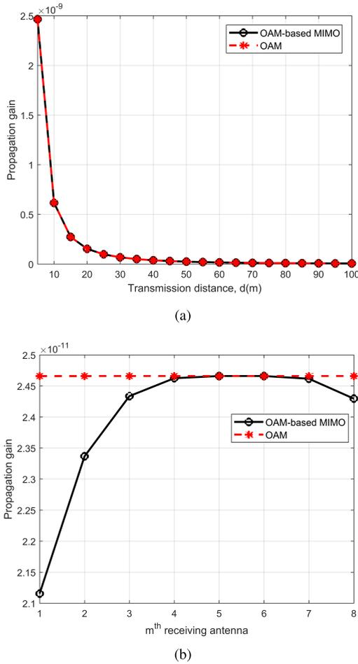
**FIGURE 2.** Propagation gains inside and outside the circle region for the OAM-based MIMO and the conventional OAM wireless channel models. (a) Propagation gain inside the circle region; (b) Propagation gain outside the circle region.
