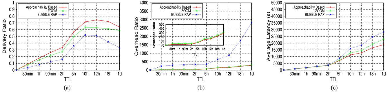
Fig. 4. Simulation results of (a) delivery ratio, (b) overhead ratio, and (c) average latency on San Francisco Cabspotting with RSUs being deployed in a dense traffic area.
