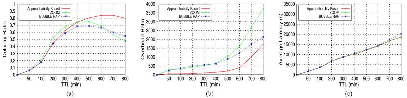
Fig. 7. Simulation results of (a) delivery ratio, (b) overhead ratio, and (c) average latency on Shanghai Taxi Movement with RSUs being deployed in a dense traffic area.
