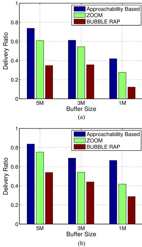
Fig. 12. Impact of buffer size on delivery ratio for (a) test on San Francisco Cabspotting and (b) test on Shanghai Taxi Movement.
