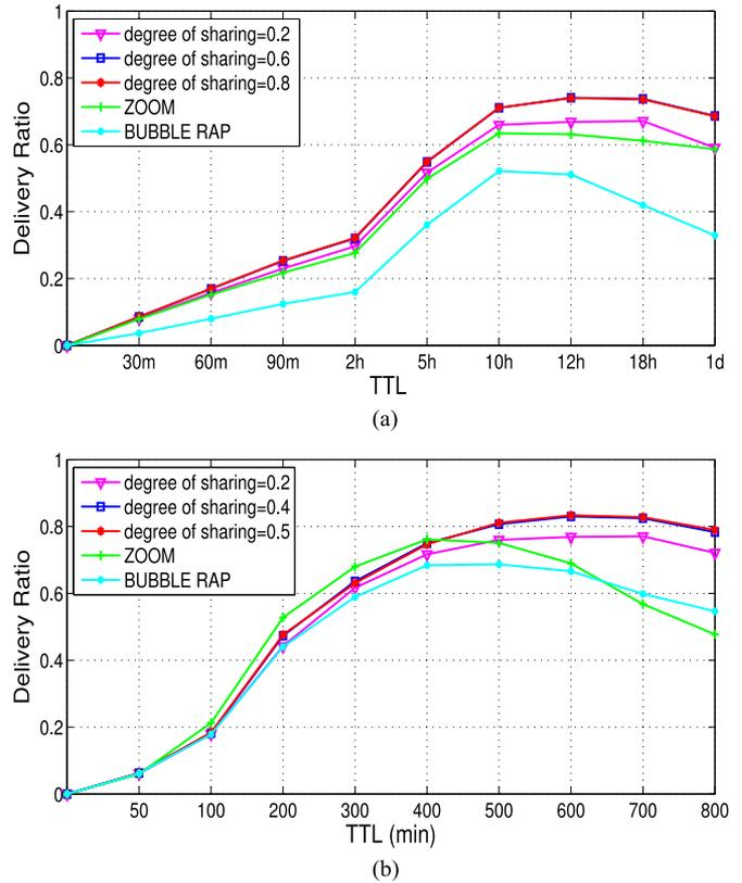
Fig. 13. Impact of degree of sharing on delivery ratio for (a) test on San Francisco Cabspotting and (b) test on Shanghai Taxi Movement.
