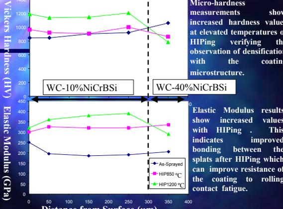
Micro-hardness measurements show increased hardness values at elevated temperatures of HIPing verifying the observation of densification with the coating microstructure.
