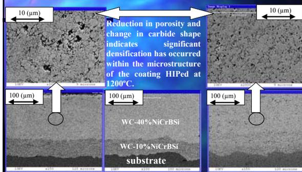
Reduction in porosity and change in carbide shape indicates significant densification has occurred within the microstructure of the coating HIPed at 1200°C.
