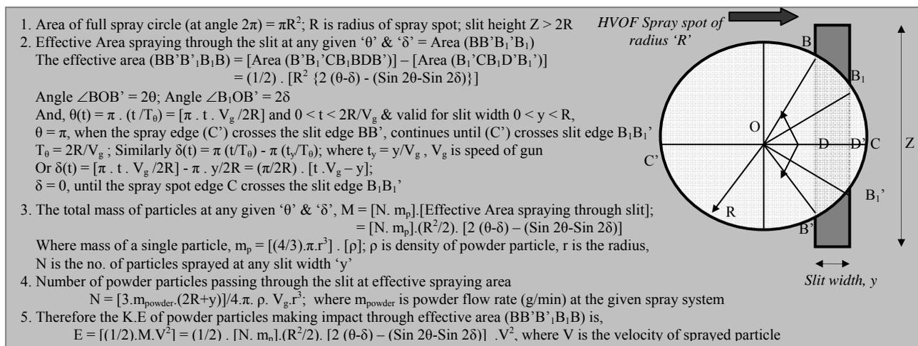
Fig. 8. Geometric model for total particle kinetic energy passing through slit.
