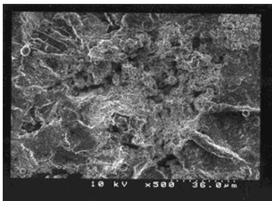
Fig. 4. Single WC-10Co-4Cr powder impact: splat located in valley on grit blasted surface, i.e. interlocking
