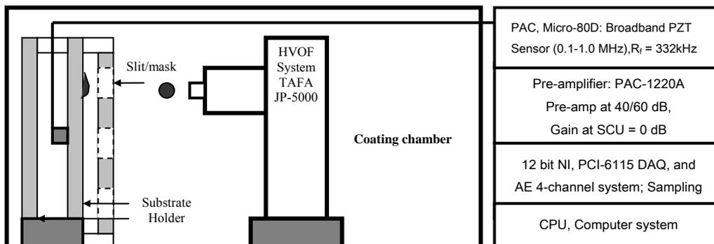
Fig. 1. Block diagram of the HVOF and AE experimental set-up with masking sheet
