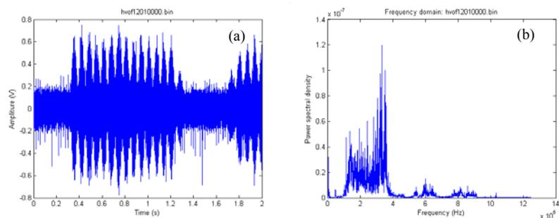
Fig. 5. AE signal (a) amplitude and (b) frequency spectrum, recorded during HVOF full spraying (both flame and powder) onto substrate through slit-A at 500 mm/sec, and pressure P1
