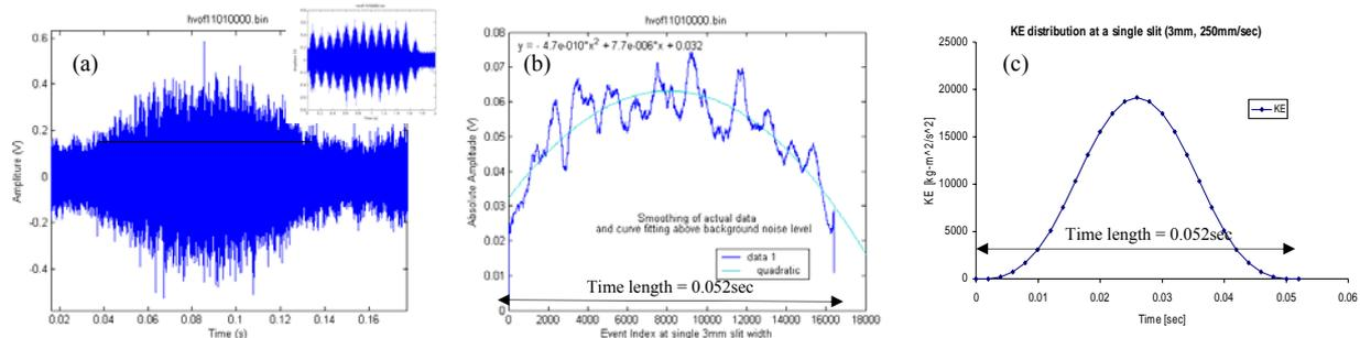
Fig. 9. (a) AE signal at a single slit of width  $3\text{mm}$  when HVOF sprayed at  $250\text{mm}/\text{sec}$  gun speed (see inset: full AE signal), (b) Curve fitting done on smoothed AE data of the absolute amplitude of (a), and (c) SPRAE model: Kinetic energy 'E(t)' distribution due to particle impact
