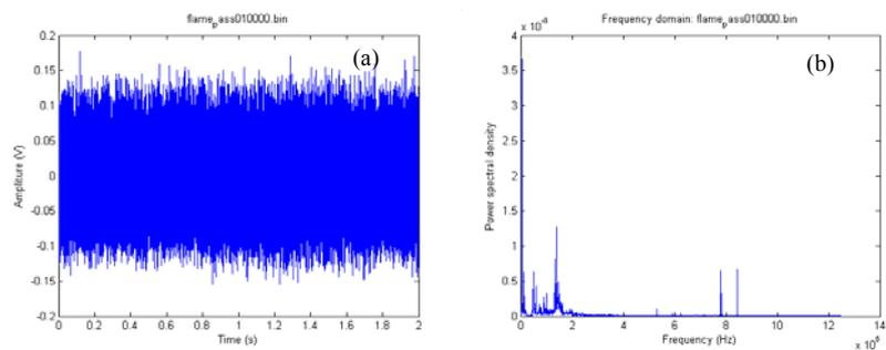
Fig. 3. AE signal (a) amplitude and (b) frequency, recorded during HVOF flame-only spraying onto substrate without powder (flame noise)
