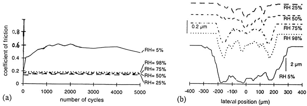
Fig. 5. Showing: (a) the evolution of the coefficient of friction with the test duration, and (b) the wear depth; on a DLC coating against alumina (normal load: 100 N; slip amplitude: 25 μm; frequency: 5 Hz); in a test atmosphere of different relative humidity [38].
