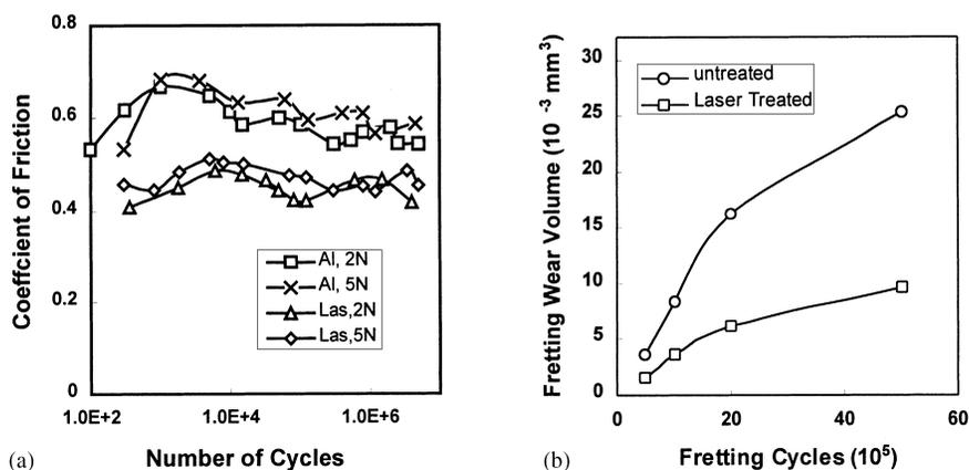
Fig. 10. Fretting wear of aluminum alloys and laser alloyed Al alloys under a slip amplitude of 100  $\mu\text{m}$  [62]: (a) coefficient of friction under different normal loads; (b) fretting wear volume under a normal load of 5 N.
