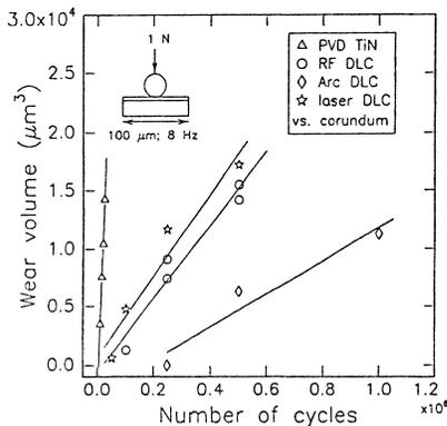
Fig. 6. Comparative fretting wear volume for a PVD TiN coating and different DLC coatings produced by different techniques (CVD, arc ion plating, laser ablating, etc.) [42].
