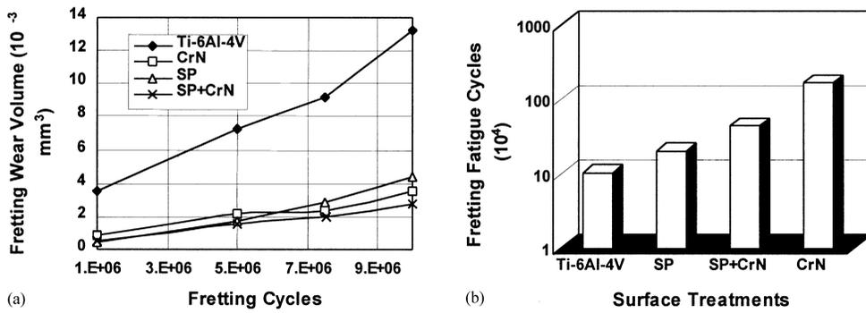
Fig. 12. Showing (a) the maximum fretting wear volume; and (b) the maximum fretting fatigue cycles; for untreated Ti–6Al–4V, shot-peened Ti–6Al–4V, IBED CrN, shot-peening + IBED CrN, under a normal load of 20 N and a slip amplitude of 50  $\mu$ m [81].
