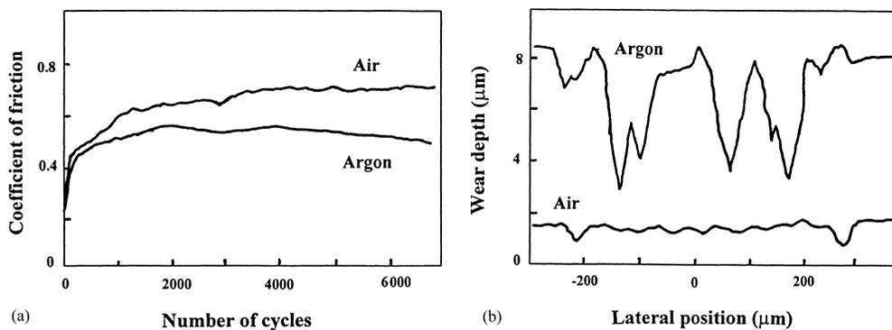
Fig. 4. Effect of argon gas and dry air on the fretting wear of a TiN coating [35]: (a) the coefficient of friction of a TiN coating in dry argon and dry air; (b) the wear depth in dry argon, which is much larger than that in dry air.
