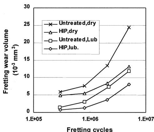
Fig. 11. Effect of hot isostatic pressing (HIP) treatment on the fretting wear behaviour of an HA coating under unlubricated and lubricated conditions under a normal load of 5 N and a slip amplitude of 100  $\mu\text{m}$  [76].
