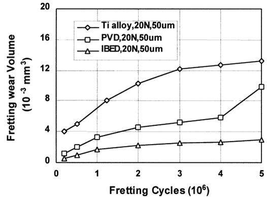
Fig. 8. The fretting wear volumes for an IBED CrN film (1  $\mu\text{m}$ ), PVD CrN film (1  $\mu\text{m}$ ) and Ti–6Al–4V substrate under the fretting conditions of 20 N and 50  $\mu\text{m}$  [56].
