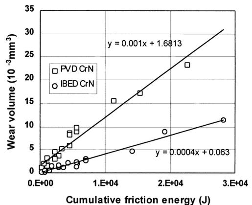
Fig. 9. Evolution of the measured wear volume on IBED CrN and PVD CrN films as a function of the cumulative friction energy [56].
