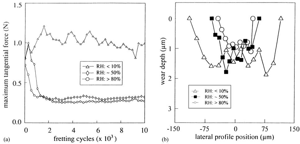
Fig. 3. Effect of the relative humidity on the fretting wear of TiN coating: (a) the evolution of the maximum tangential force with the fretting test duration on a TiN coating under different relative humidities; (b) position–depth profiles of fretting scar induced on a TiN coating by a corundum counterface after 10 000 cycles (normal load: 2 N; amplitude: 100  $\mu\text{m}$ ; frequency: 10 Hz) [33].
