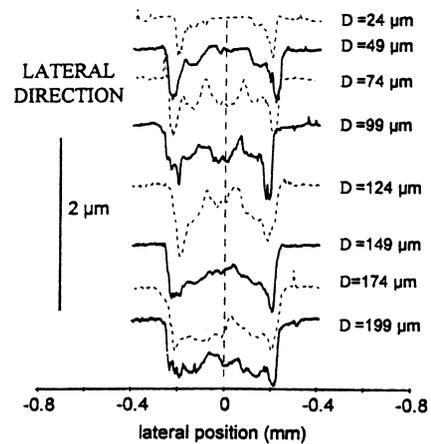
Fig. 2. Effect of the slip amplitude on the fretting wear volume of a PVD TiN coating [32].
