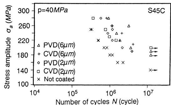
Fig. 7. Fretting fatigue characteristics of different coatings on a S45C steel specimen [44].
