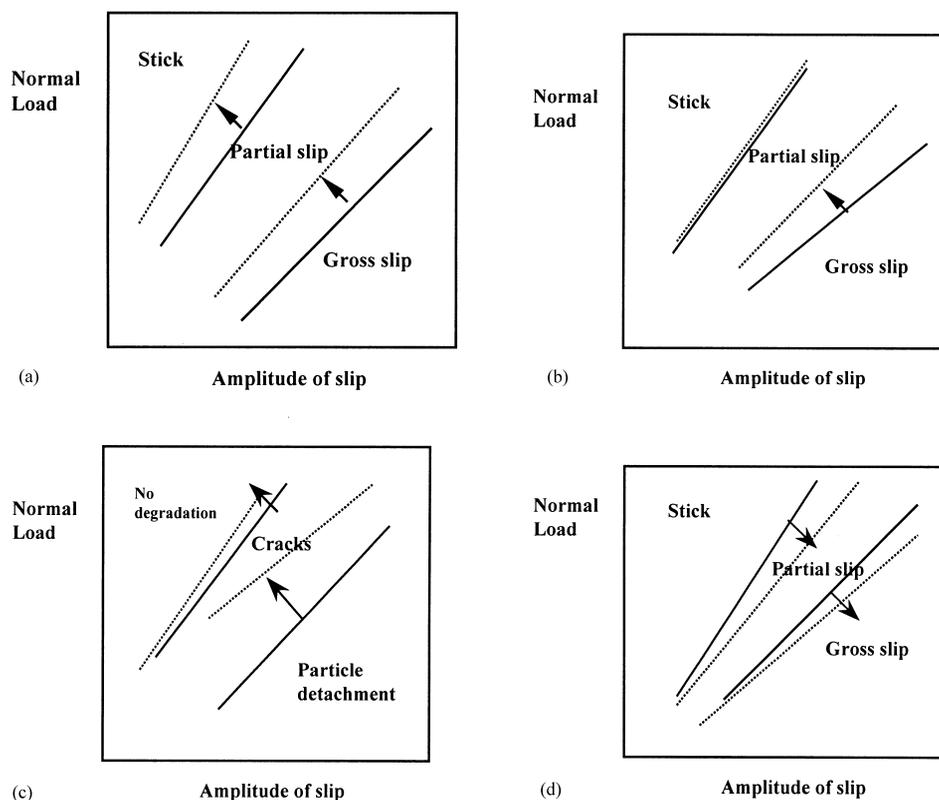
Fig. 13. Effect of surface modification technologies on the changes in fretting maps: (a) effect of decrease in the coefficient of friction; (b) effect of some hard coatings; (c) effect of increase in compressive stress; and (d) effect of increase in surface roughness.
