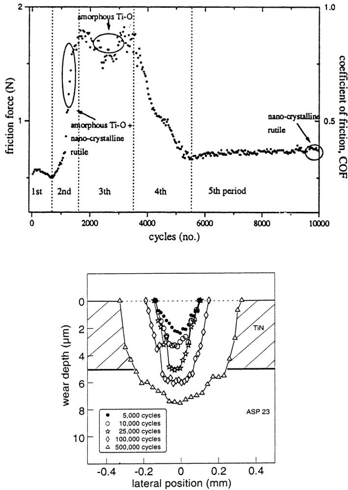
Fig. 1. Showing (a) the evolution of the friction force as a function of the number of fretting cycles during fretting tests on a TiN–corundum tribo-pair [30]; (b) the progress of fretting damage on TiN coatings on nitrided ASP 23 tool steel, where position–depth profiles were obtained by laser profilometry along a track normal to the fretting direction in the centre of the fretting scar [31].
