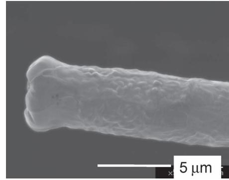
Fig. 10. SEM photograph of a blowup tip, showing a rounded structure which was caused by thermal runaway and melting.
