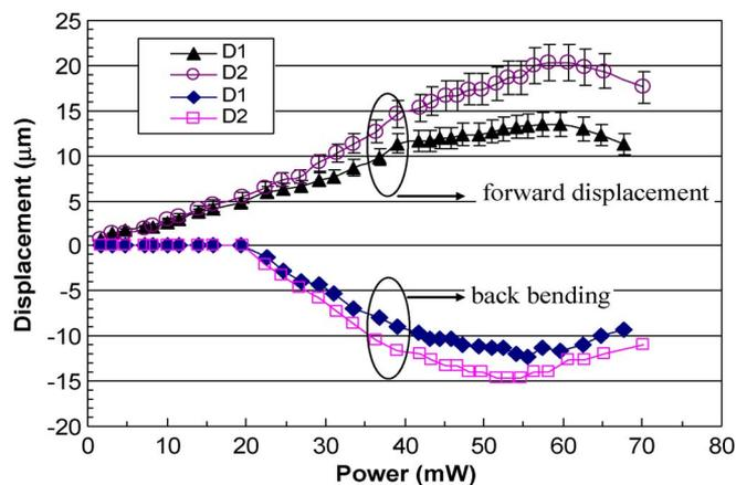
Fig. 3. Forward displacements and back bending of the Ni actuators as a function of power consumed, which were calculated from the current applied and voltage measured. The back bending appears at a current larger than 20 mA.
