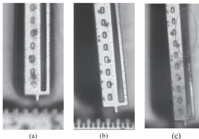
Fig. 7. Optical images of a thermal actuator show (a) the initial tip position and (b) the back bending after applying a pulse current of 54 mA and (c) burn-off followed by a high current of  $\sim 62$  mA.
