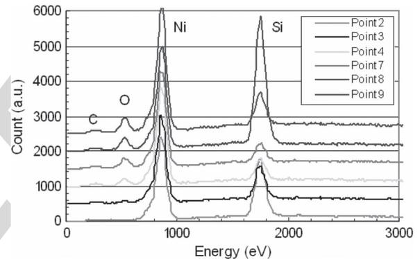
Fig. 11. EDX spectra from the surface of a hot arm after thermal stress at 55 mA for 3 min. As approaching the middle of the arm, the oxygen signal becomes much stronger.
