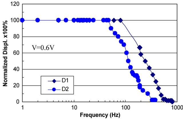
Fig. 5. Dependence of normalized displacements of Ni actuators on the frequency. The displacement remains unchanged at a frequency smaller than 40–100 Hz; it decreases with increasing the frequency and diminishes at a frequency higher than 300–700 Hz.
