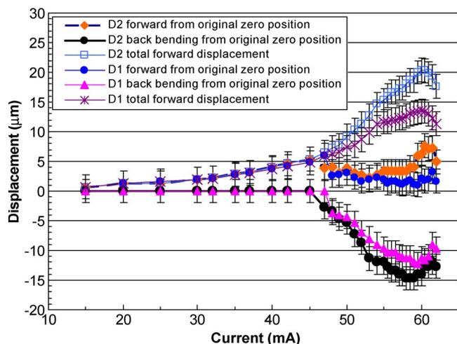
Fig. 2. Displacements of the Ni actuators as a function of pulsed current. The current pulsewidth was 0.1 s. Device D1 and D2 have different Ni thicknesses of 3 and 4  $\mu\text{m}$ .
