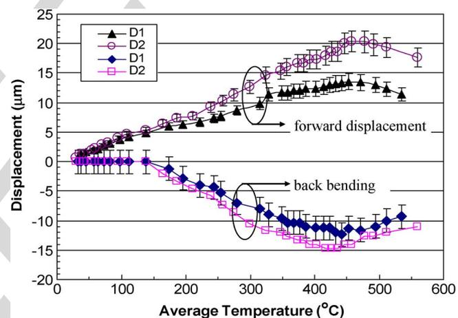
Fig. 4. Forward displacements and back bending as a function of average temperature extracted for two thermal actuators. The forward displacement is almost proportional to the average temperature. The back bending appears at an average temperature larger than 140  $^{\circ}\text{C}$ .
