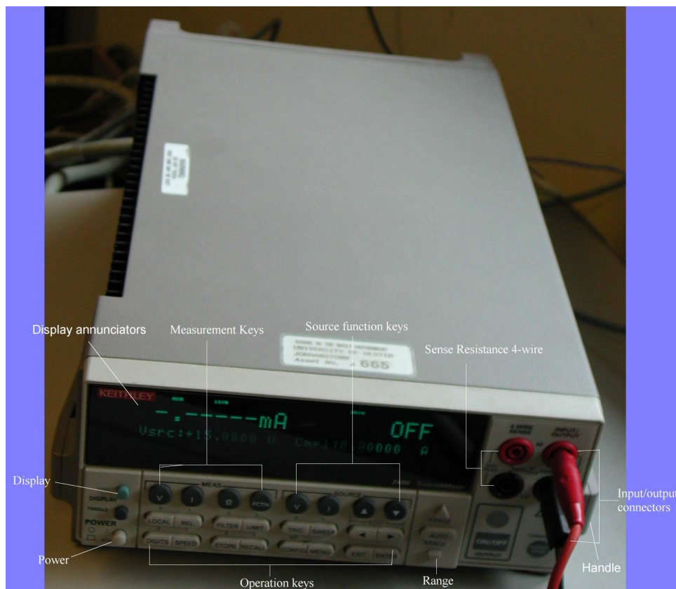
Figure B.1.1.1 Model 2400 Keithley source meter for sourcing and sinking voltage/current for the test device.
