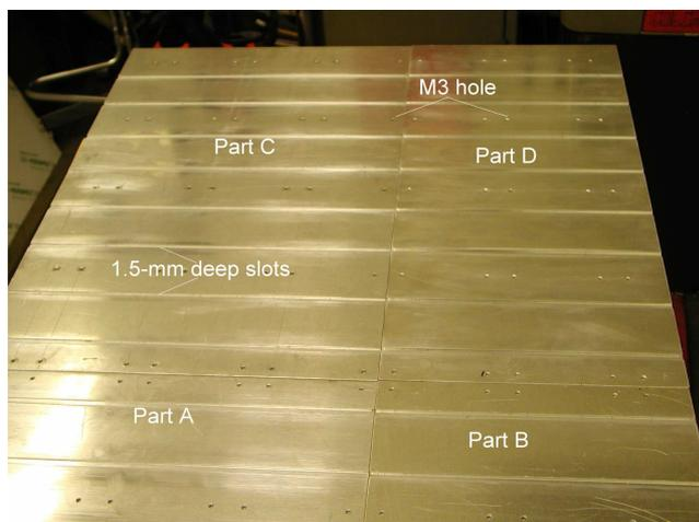
Figure 3.5.3.1 Construction of the rear aluminium back plate. Four aluminium plates of 3mm thick were screwed to a single aluminium plate.
