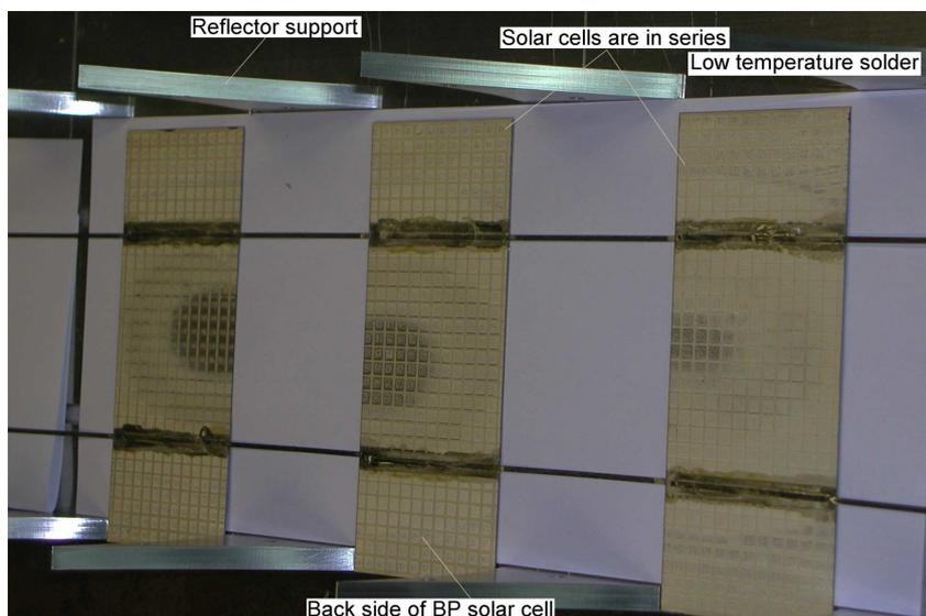
Figure 3.5.4.3 Alignment and interconnection of individual solar cells in series. The solar cells were located between two reflector supports during soldering to ensure their accurate positioning.
