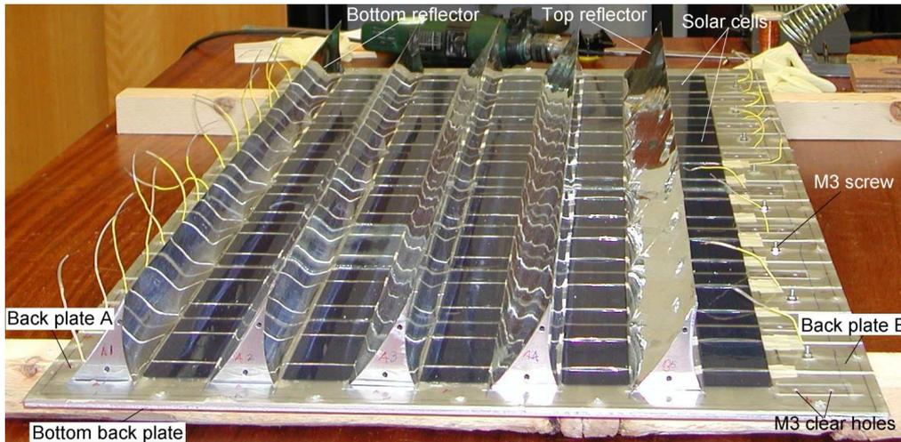
Figure 3.5.7.1 Placement of detachable reflector troughs on the aluminium back plate with the encapsulated PV cells.
