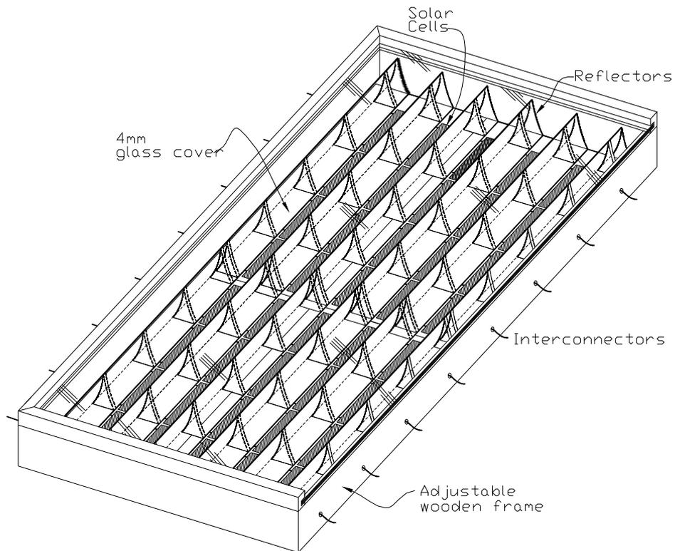
Figure 3.6.2.2 The full Asymmetric compound parabolic photovoltaic concentrator system.
