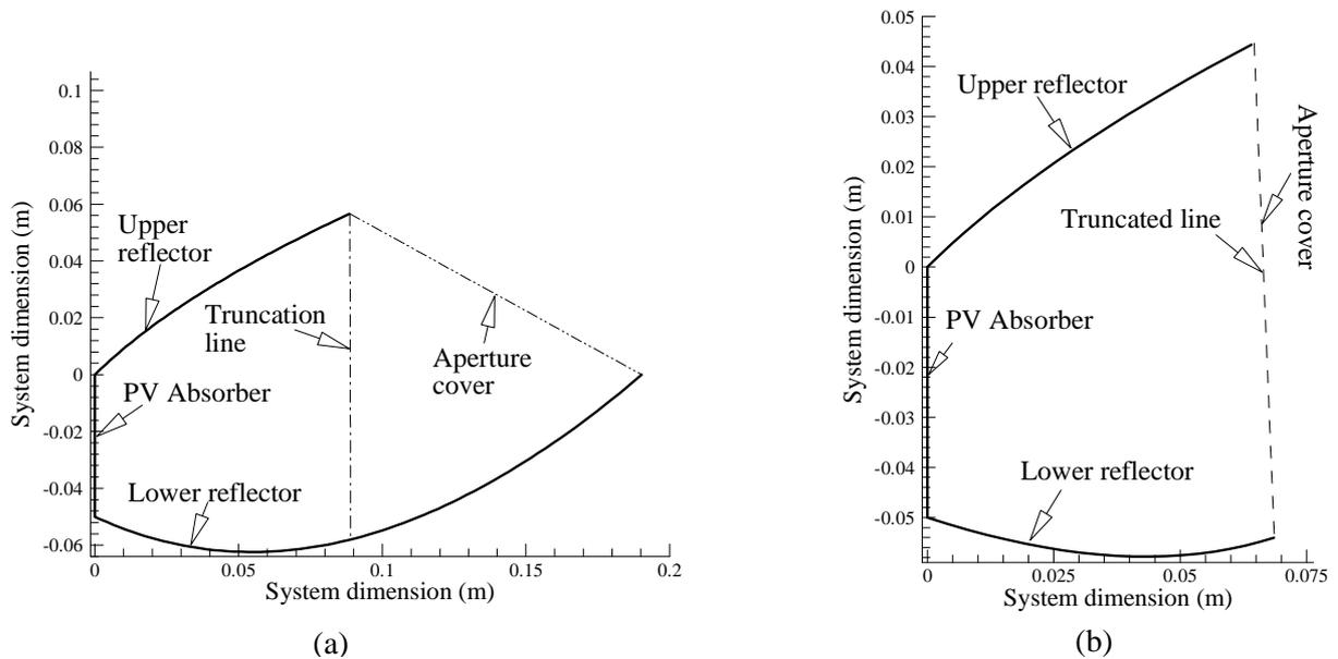
Figure 3.4.2.1 Computer generated asymmetric compound parabolic reflector profile (a) untruncated system (pointing out the truncation line) (b) truncated system.
