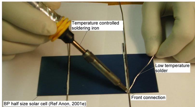
Figure 3.5.4.2 Soldering of front connection of solar cells.
