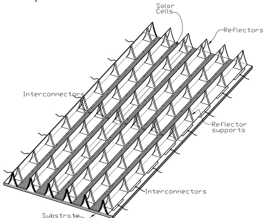
Figure 3.5.7.2 The ACPVC-50 system used for outdoor experimental characterisation without the wooden frame or cover glass.
