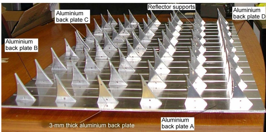
Figure 3.5.3.3 Reflector supports placed on the rear aluminium back plate.
