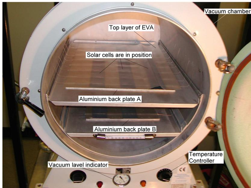
Figure 3.5.6.2 Encapsulation of solar cells with EVA in a vacuum oven.
