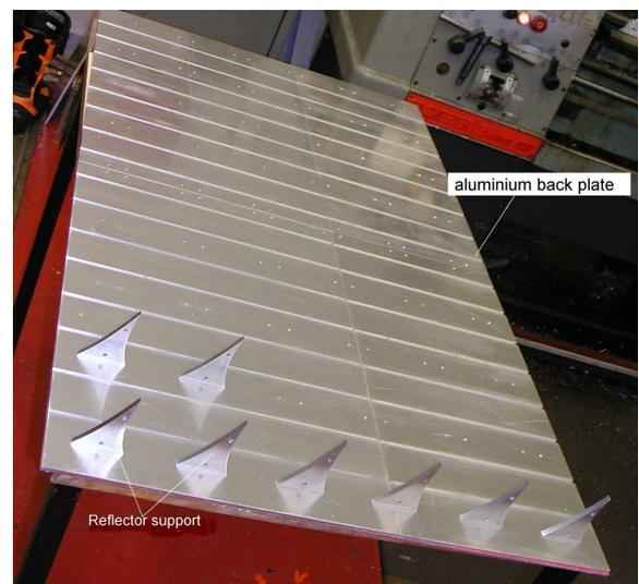
Figure 3.5.3.2 Locating reflector supports on to the rear aluminium back plate.
