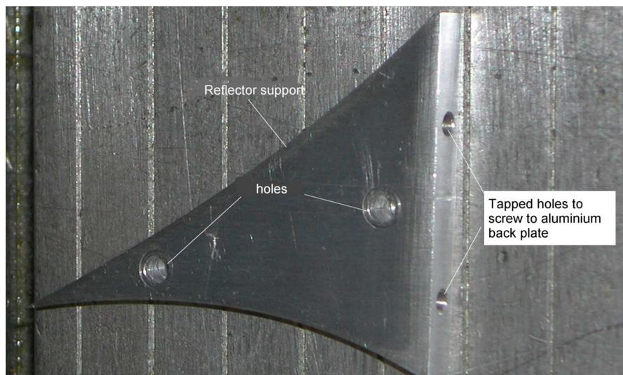
Figure 3.5.2.1 A 6-mm thick aluminium reflector support.
