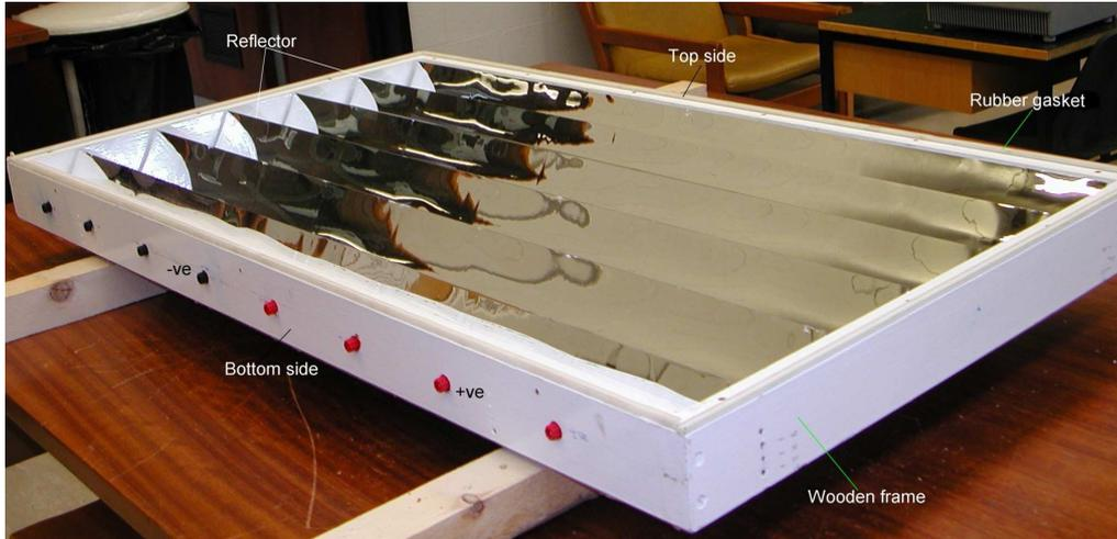
Figure 3.5.8.1 Asymmetric compound parabolic photovoltaic concentrator with wooden frame.
