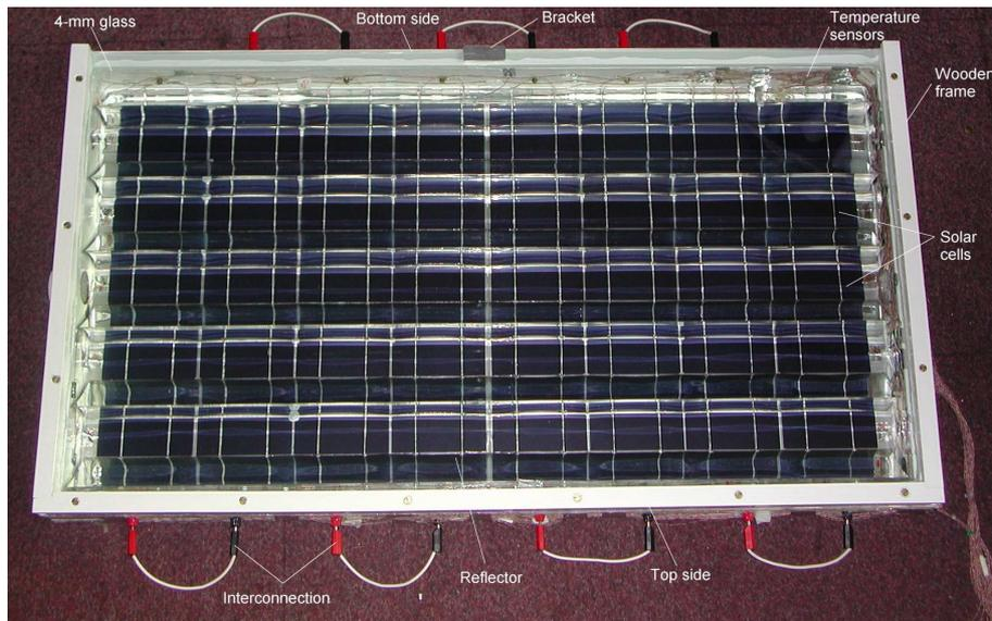
Figure 3.6.2.5 The plan view of the 2<sup>nd</sup> ACPPVC-50 with temperature sensors inside the system.
