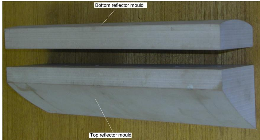
Figure 3.5.1.1 Top and bottom reflector mould.
