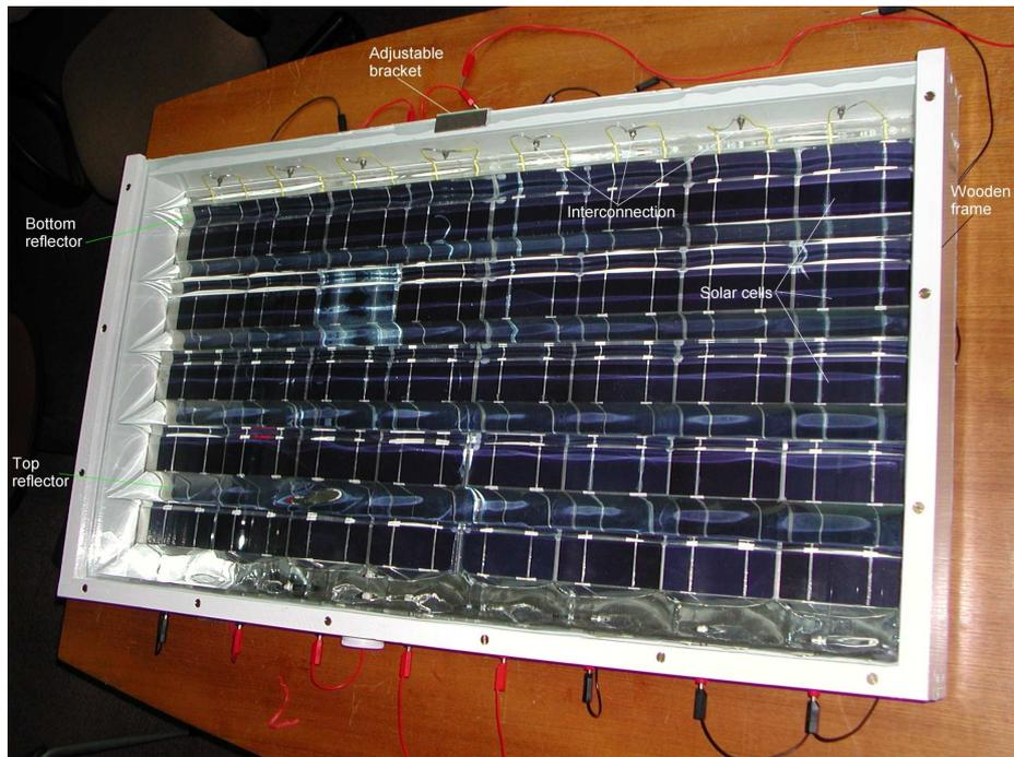
Figure 3.6.2.4 The plan view of the asymmetric compound parabolic photovoltaic concentrator used for outdoor experimental characterisation.
