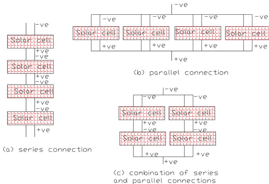
Figure 3.5.4.1 Solar cell connections (a) series connection to increase voltage (b) parallel connection to increase current (c) combination of series and parallel connections to increase current and voltage.
