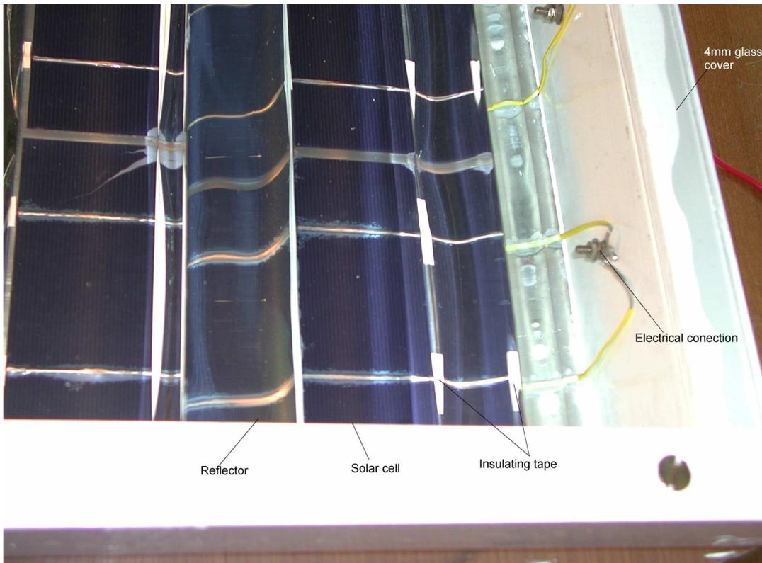
Figure 3.5.8.2 Internal electrical connections of solar cells through the wooden frame. Each series of solar cells are connected individually to each electrical connector.
