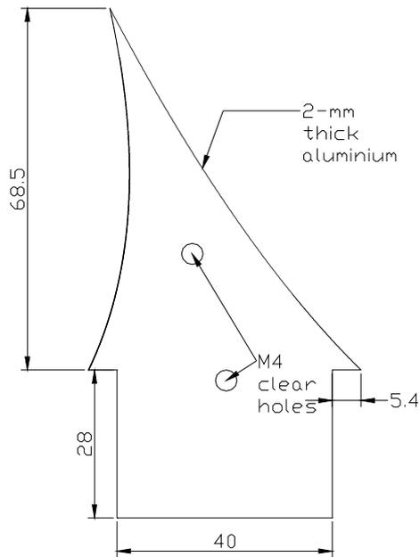
Figure 3.4.2.1.1 Aluminium reflector support for the asymmetric compound parabolic photovoltaic concentrator.
