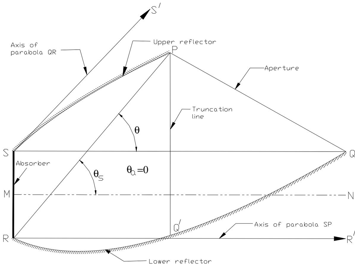
Figure 3.3.1 Asymmetric compound parabolic concentrator for building integration in the UK with acceptance-half angles of  $0^\circ$  and  $50^\circ$ .
