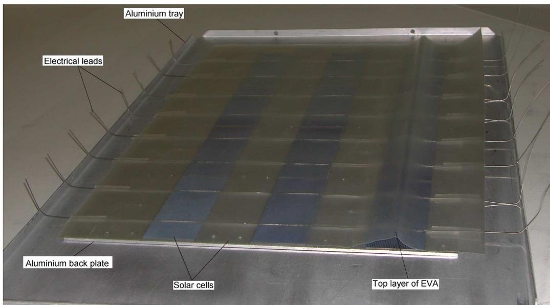
Figure 3.5.6.1 Line up of solar cells on the aluminium back plate. Individual solar cells are connected in series.
