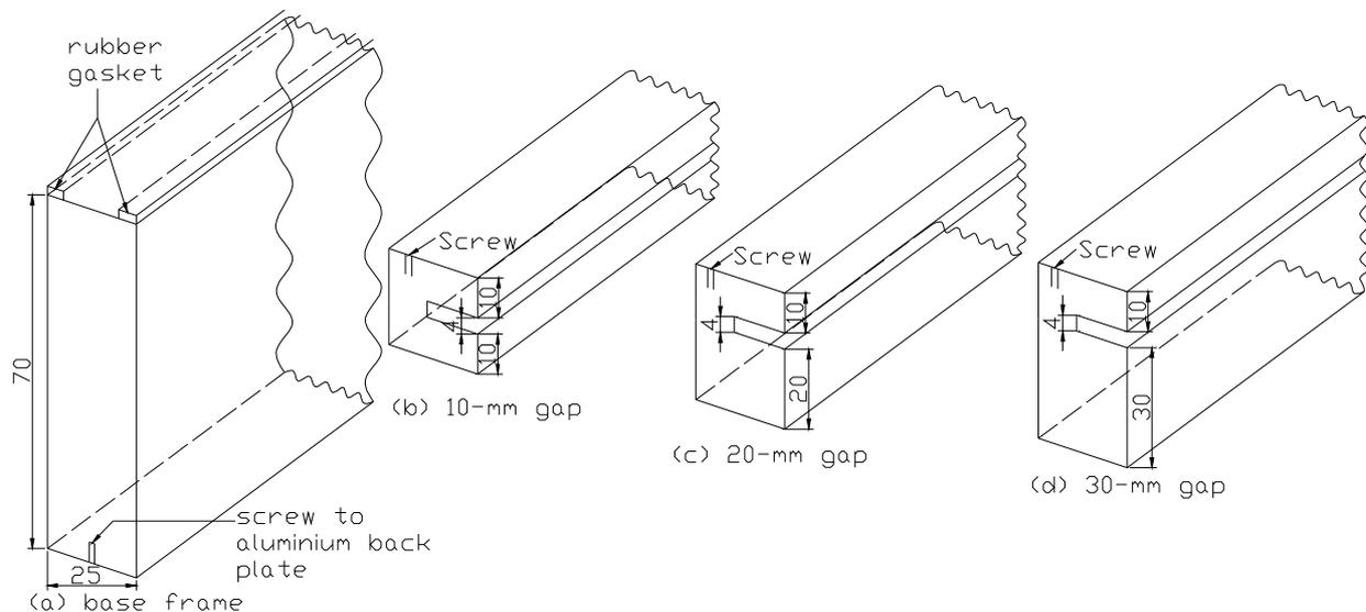
Figure 3.4.5.1 Adjustable wooden supporting frame for the ACPPVC-50 system: (a) base frame (b) top frame with 10-mm gap between reflector end and glass cover (c) top frame with 20-mm gap between reflector end and glass (d) top frame with 30-mm gap between reflector end and glass cover.
