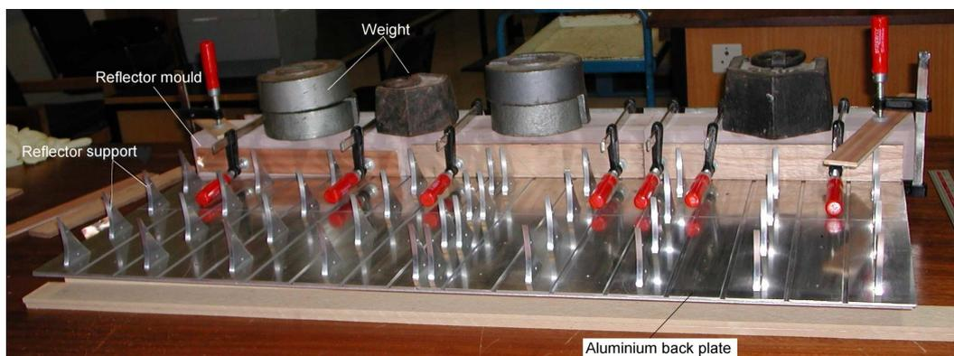
Figure 3.5.5.1 Attachment of mirror reflector to the reflector support. The mirror was attached to a 0.0003 m thick stainless steel back plate.
