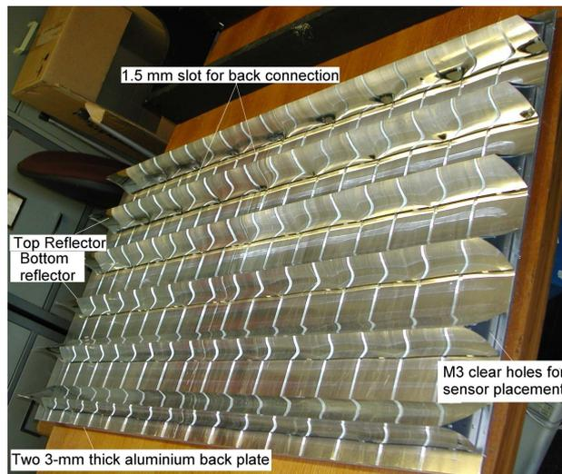
Figure 3.5.5.2 Asymmetric compound parabolic photovoltaic concentrator with mirror reflectors attached to the rear aluminium back plate.
