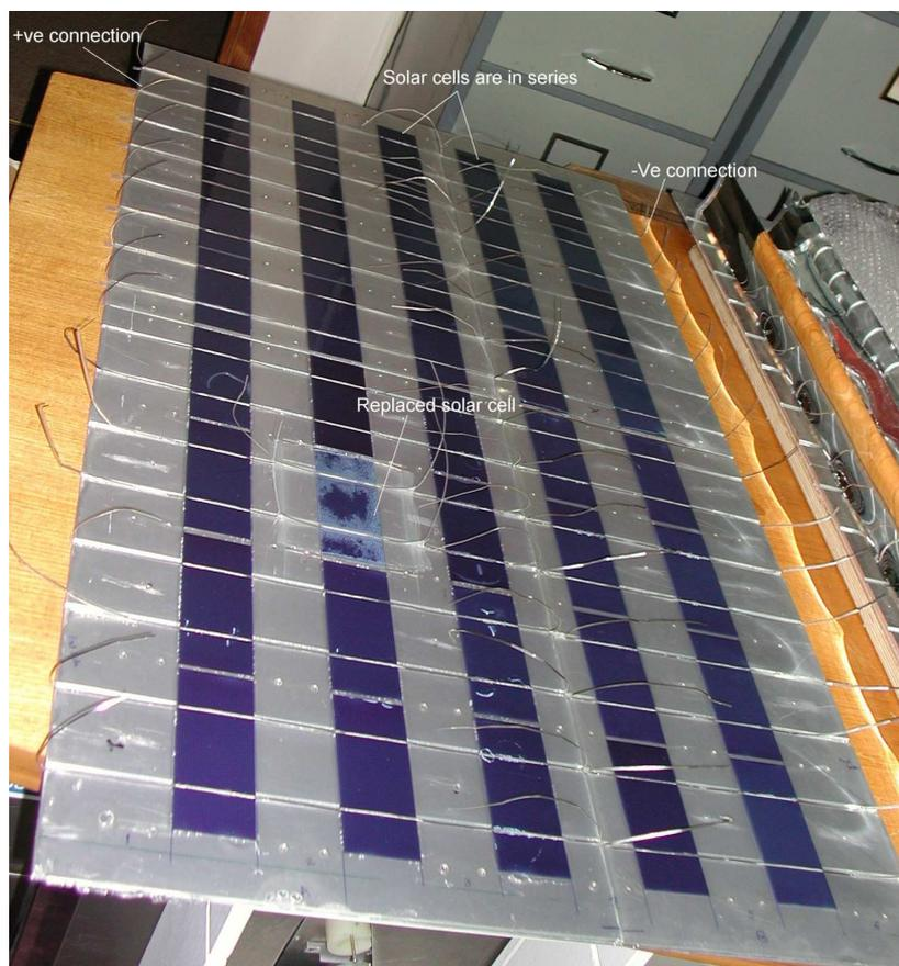
Figure 3.5.6.3 Solar cells encapsulated on to the aluminium back plate clearly showing the replaced solar cell.
