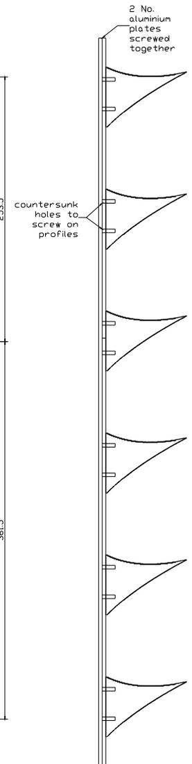
Figure 3.4.4.3 Top view of rear aluminium plate of the ACPVC-50 used for outdoor experimental characterisation.
