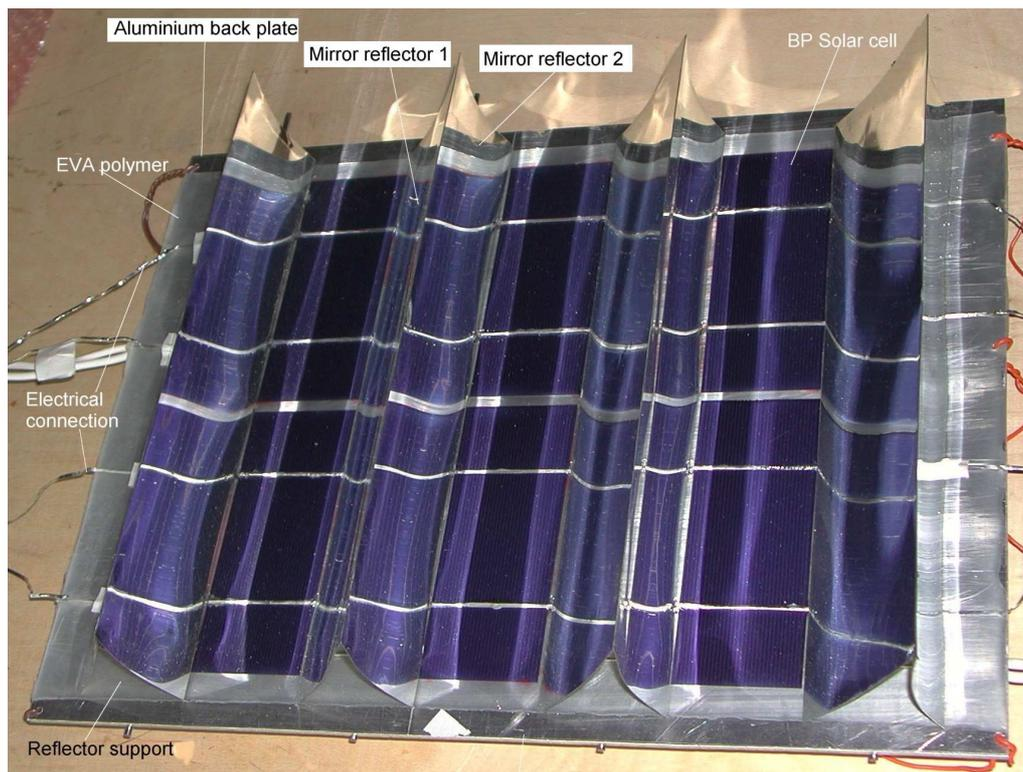
Figure 3.6.1.1 Fabricated asymmetric compound parabolic photovoltaic concentrator used for indoor experimental characterisation.
