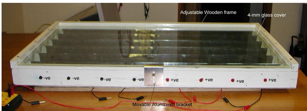
Figure 3.6.2.3 Side view of the asymmetric compound parabolic photovoltaic concentrator used for outdoor experimental characterisation.
