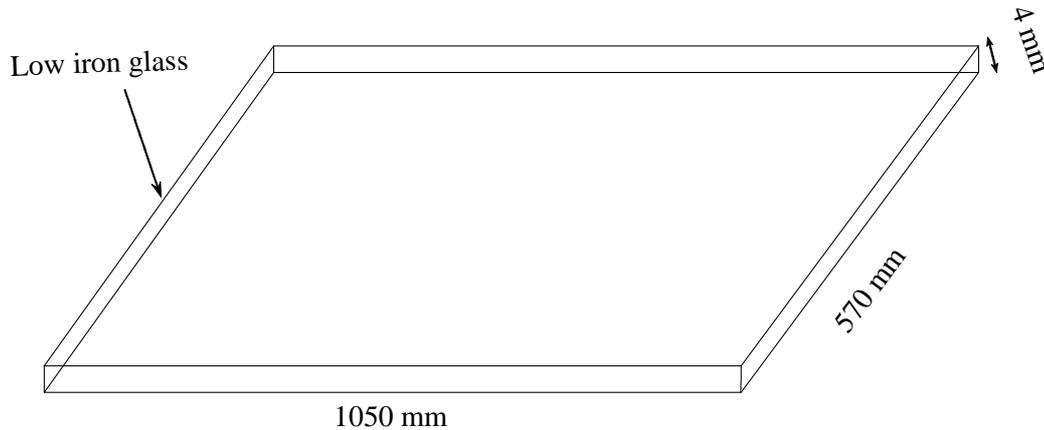
Figure 3.4.1.1 Aperture cover specification for the ACPVC-50 system.
