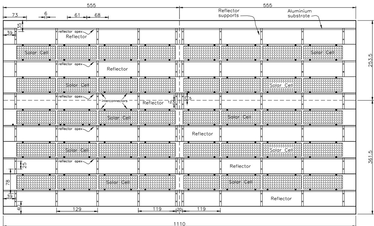
Figure 3.6.2.1 Top view of the ACPVC-50 system used for outdoor experimental characterisation.
