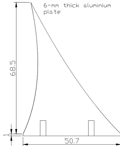
Figure 3.4.2.1.2 Modified reflector support design for outdoor experimental characterisation of the ACPVVC-50.
