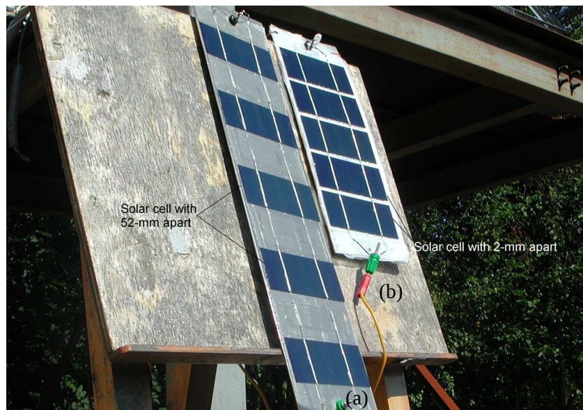
Figure 7.4.1 Non-concentrating solar panels with (a) 52-mm (b) 2-mm tab spacing between individual solar cells without EVA and no glass cover.
