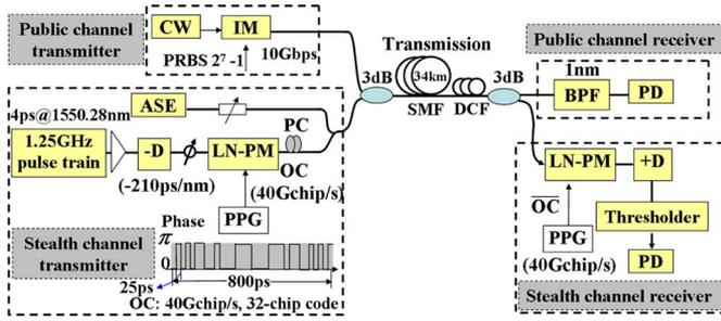
Fig. 1. Experimental setup of the stealth OCDMA signal transmission over public WDM channel.
