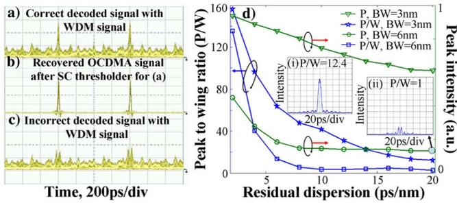
Fig. 4. (a) Correct decoded signal with WDM channel; (b) recovered stealth signal after threshold; (c) incorrect decoded signal with WDM channel; and (d) peak-to-wing ratio (left) and peak intensity (right) of decoded waveform versus RD for different BW. Insets (i) and (ii) are the decoded waveforms for BW = 3 nm and BW = 6 nm with RD = 20 ps/nm.
