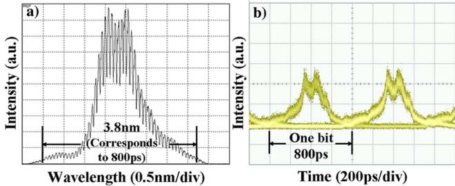
Fig. 2. (a) Spectrum and (b) waveform of the broadened pulse after the LCFBG.
