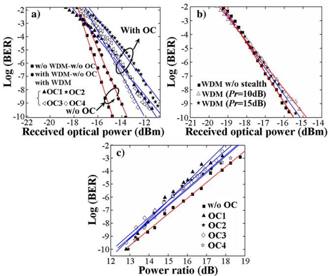
Fig. 5. (a) BER for stealth OCDMA channel with and without OC; (b) BER for public WDM channel; and (c) BER versus power ratio for stealth channel.
