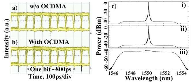
Fig. 3. Eye diagram of public WDM channel without (a) and with (b) stealth OCDMA signal; (c) spectrum of public WDM channel without (i) and with (ii) OCDMA signal and (iii) spectrum of stealth channel with ASE noise.
