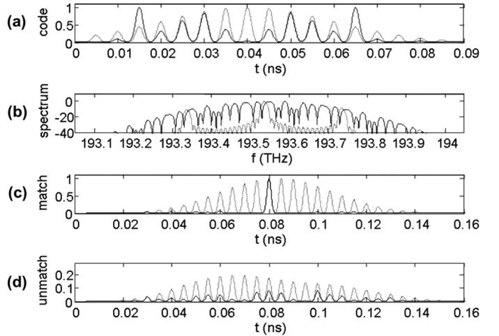
Fig. 3. (a) Intensity of the code; (b) spectral content; (c) auto-correlation; (d) cross-correlation. Continuous line refers to a spectral-phase code with random phase and dotted line to a PSK code.
