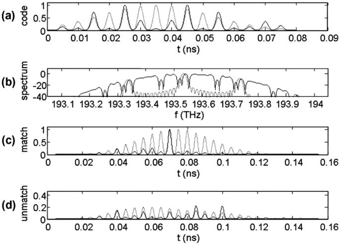
Fig. 4. (a) Intensity of the code; (b) spectral content; (c) auto-correlation (d); cross-correlation. Continuous line refers to a spectral-phase code with  $m$ -sequence phases and dotted line to a PSK code.
