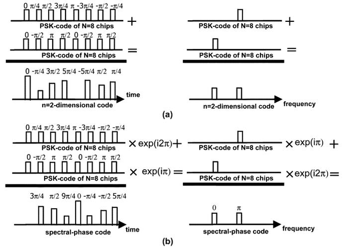
Fig. 1. Schematic of the code generation in time and frequency domains (a) multidimensional code ( $n = 2$ ); (b) spectral-phase code.
