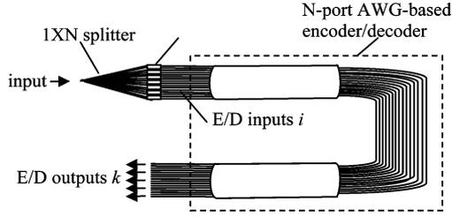
Fig. 2. Architecture of the spectral-phase E/D consisting of an AWG, an input splitter, and an array of phase shifters.
